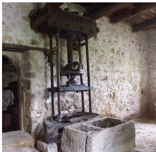
Figure 7 Olive press (Lever, screw & axle)
