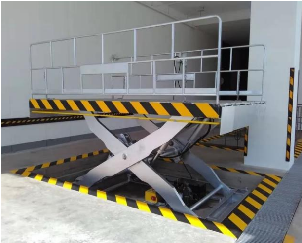
Figure 9 Scissor lift (Lever, screw, toothed bar)
