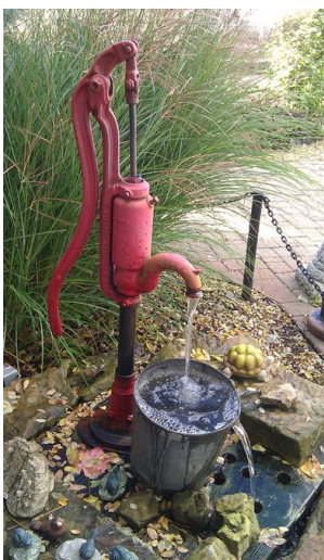
Figure 6 Manual water pump (Lever and axle)
